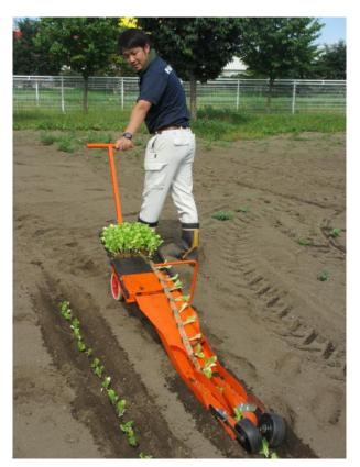
The easy-to-use  $Hippari-kun \,^{\text{TM}}$  Transplanter, specially designed to be used with  $CHAINPOT^{\text{TM}}$ , in action. The condition of the transplanting process, as well as post-transplant seedlings, are visible.
